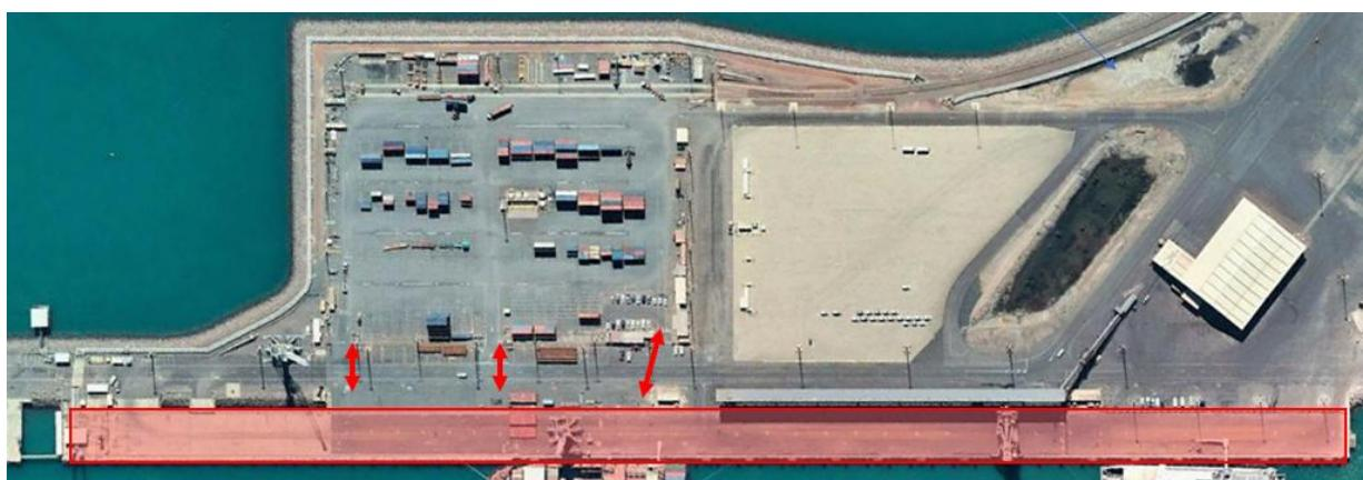
The transport of 40-foot Containers, break bulk and out of gauge cargo to and from the common user yard and adjacent laydown areas using reach stackers and conventional forklifts is authorised to take place directly from the wharf to the common user precinct and along the wharf deck only. Above is the depiction of approved transport route, when break bulk and out of gauge operations occur, this area adjacent to the wharf road must be traffic managed by the respective stevedore.
