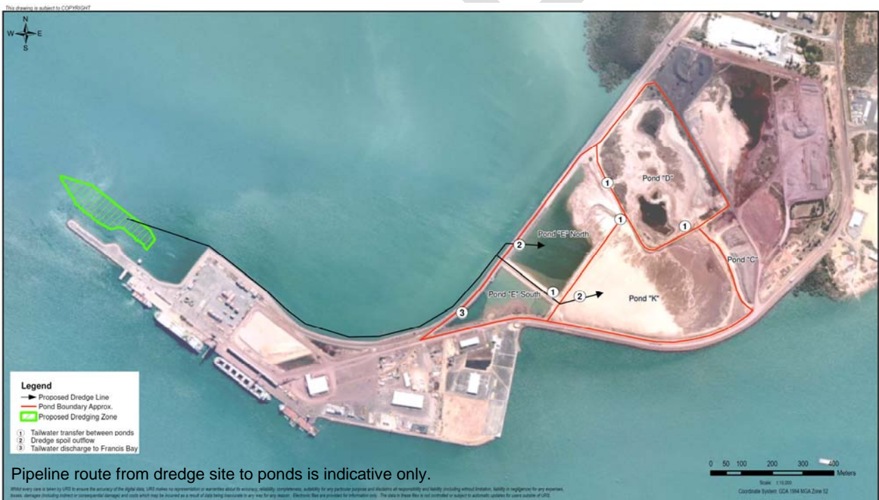
Figure 2-2 Placement of dredge spoil into EAW Ponds
