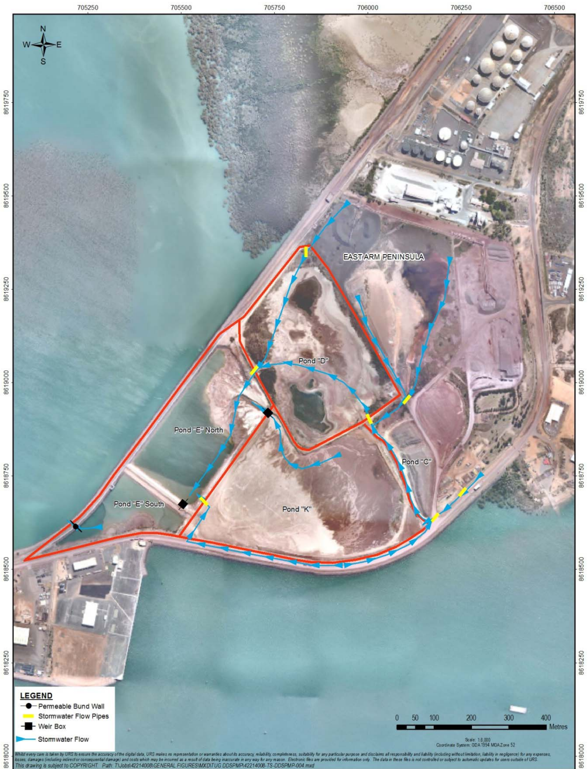
Figure 2-3 Stormwater flow paths through EAW pond system
