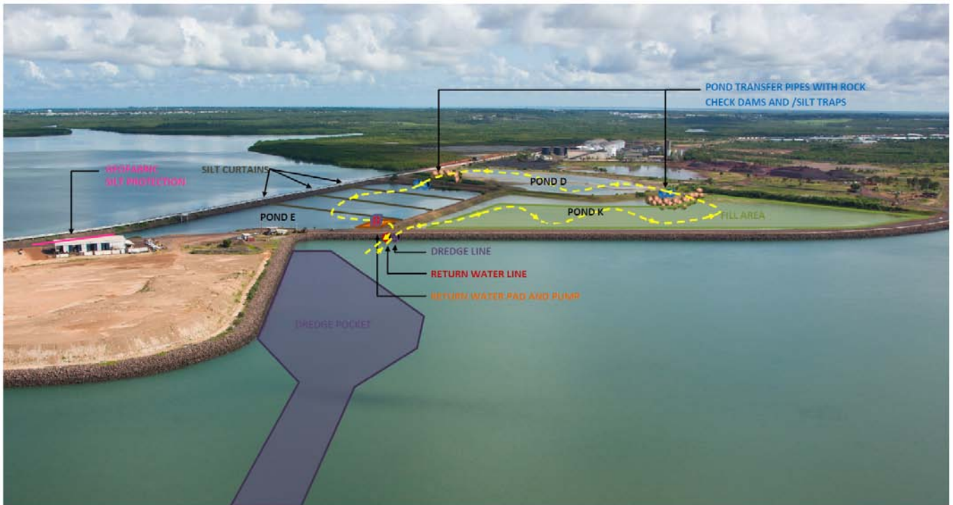
Figure 3 – Pond System and Decant Water Flow
